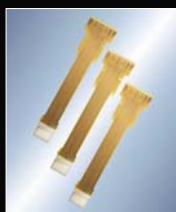
Newly-developed 0.7-inch full HD D-ILA device
