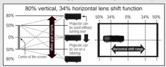
\*The vertical and horizontal lens shifts cannot be set to maximum values at the same time
