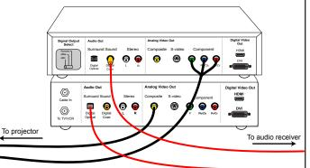
Connect audio and video cables to sources. Connect audio cables to speaker system.
