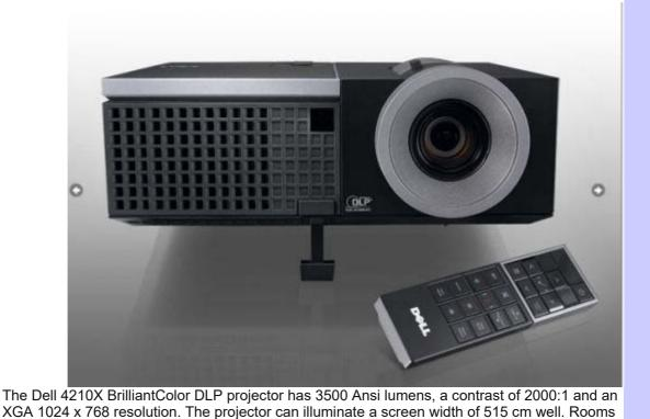
with residual light can be created by the projector with a smaller image width, max. 343 cm is
