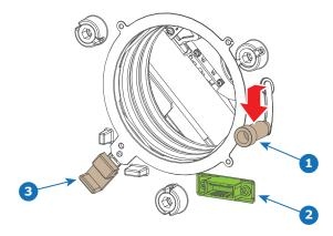
2. Gently insert the projection lens in the lens holder while aligning the lens connector with the electrical socket (reference 2) until a click is heard.
