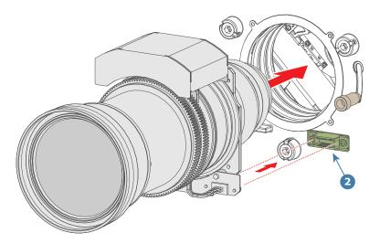
**3.** Secure the lens by sliding the primary lens lock handle to the "locked" position.
