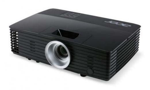
The standard portable P1285B TCO new 3D DLP has 3300 Ansi lumens, a contrast of 20000:1 and an XGA 1024 x 768 resolution. The lamp life is specified by the manufacturer as 10000 hours, which converts to over 13.7 years at 2 hours per day. Due to the brightness of 3300 Ansi lumens, a picture width of 500 cm is possible. In room light, the picture should be max. 333 cm
