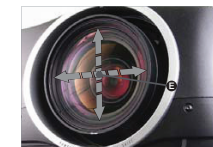
D: Lens shift (operated from back)
